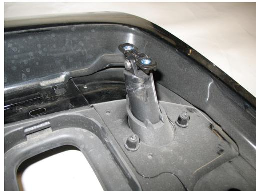
6 Remove the circlip holding the pivot pin and remove the nut plate from the top of each plastic piston. For installation of Getty Design's Aero Cab, GT2 Insert for 997 or Pedestal Wing, no further disassembly of the decklid is needed. The pistons continue to function inside of the insert.
