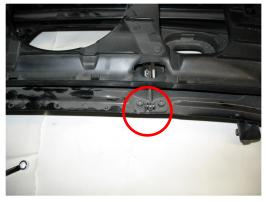
4 Remove the two 6 mm hex head bolts holding each hinge to the front of the steel decklid
