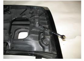
3 Remove the two 6mm bolts holding the under tray to the top of each piston.
