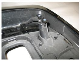
6 Remove the circlip holding the pivot pin and remove the nut plate from the top of each plastic piston. For installation of Getty Design's Aero Cab, GT2 Insert for 997 or Pedestal Wing, no further disassembly of the decklid is needed. The pistons continue to function inside of the insert.
